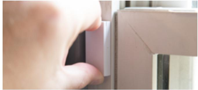
**Step 4:** Place the second, smaller sensor on the window.
