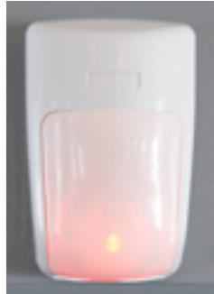
For the next three minutes the sensor will be in a "Walk Test" mode - a red LED will light up to indicate motion.
