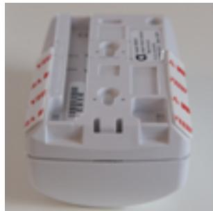
**Step 4:** Clean the mounting surface ideally with rubbing alcohol. Let the surface dry. Press and hold the motion sensor into the corner or wall. Press firmly and hold for at least 10 seconds to ensure a strong connection.
