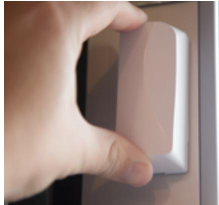
**Step 4:** Open the garage door fully so the sensor is "upside down" and check your SCW Shield app to confirm it shows as open.
