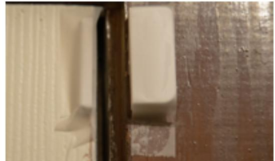
**Step 3:** Once you've selected a good spot - clean the surface area of the door, ideally with rubbing alcohol. Be sure that the surface temperature is above 50 degrees. Dirty or cold surfaces may cause the sensor to fall off, causing a false alarm. After cleaning be sure to let the surface dry before placing sensors.
