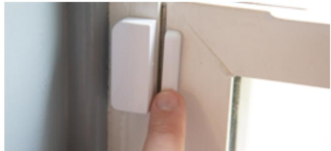
**Step 5:** Test the sensor by opening the window and monitoring the SCW Shield app. When the window is open it should register as open on the app.
