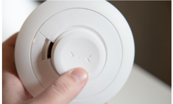
**Step 5:** Put the alarm back on the alarm base by lining up the line on the base with the line on the alarm and twisting to lock into place.
