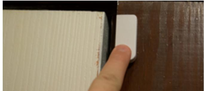
**Step 5:** Place the second sensor on the door. Monitor your SCW Shield app to make sure the contact is coming up as closed before securing it with the double sided tape. Press and hold the sensor on the door for 10 seconds to ensure a strong connection.
