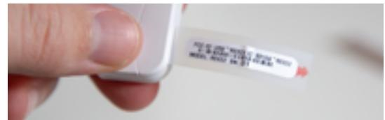
**Step 2:** Once you've selected a good spot - clean the surface area of the door, ideally with rubbing alcohol. Be sure that the surface temperature is above 50 degrees. Dirty or cold surfaces may cause the sensor to fall off, causing a false alarm. After cleaning be sure to let the surface dry before placing sensors.
