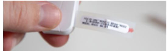
**Step 2:** Door sensors should be placed on the top of the door for best signal strength.
